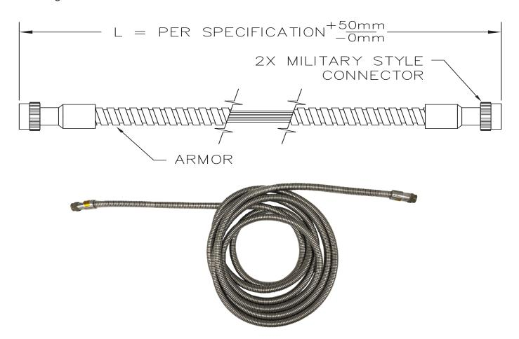
The Intank Cable includes two Military Style connectors at each end that would connect to either a six pin or ten pin High Pressure Feedthrough. The armor cable helps protect the MX8031 triaxial cables from the active flow stream in the cryogenic fluid. The Intank Cable includes 3 to 5 MX8031 Extension Cables with standard lengths of 5100mm and 4000mm. Other lengths available upon request.
