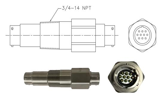
The 10-Pin High Pressure Feedthrough is rated for 150 bar (2175 psi) at -170°C (-274°F) and fits between the above listed cables, for 4 and 5 Probe Proximity Systems.
