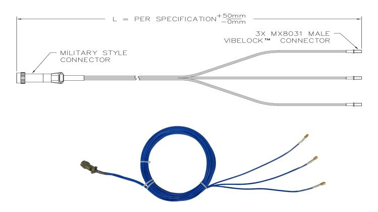
The Secondary Transition Cable connects the high pressure feedthrough to the MX2033 Proximity Driver or the MX2034 Proximity Transmitter. The Secondary Transition cable can be constructed from two to five individual MX8031 Extension Cables with standard lengths of 5200mm and 11558mm, all with male Viblock™ connectors. Other lengths are available upon request.
