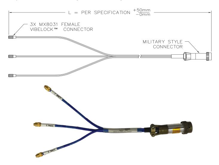
The Primary Transition Cable connects the standard MX8030 probes observing position or speed to the first bulkhead transition or feedthrough. The Primary Transition cable can be constructed from two to five individual MX8031 Extension Cables in standard lengths of 250mm, 400mm and 500mm, all with female Viblock™ connectors. Other lengths are available upon request.
