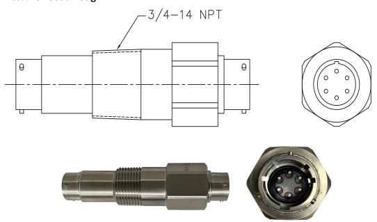
The 6-Pin High Pressure Feedthrough is rated for 150 bar (2175 psi) at -170°C (-274°F) and fits between the above listed cables for 2 and 3 Probe Proximity Systems.
