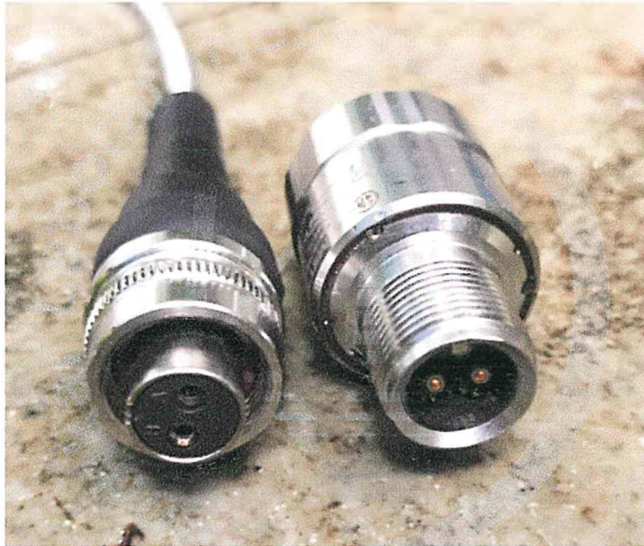
Picture2: No ingress of powder & water found
