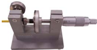
Figure 5 - Micrometer assembly or “static calibrator”
