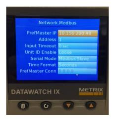
1.4 Write down the IP Address of DATAWATCH from Network\Interface menu for later use by Modbus server
