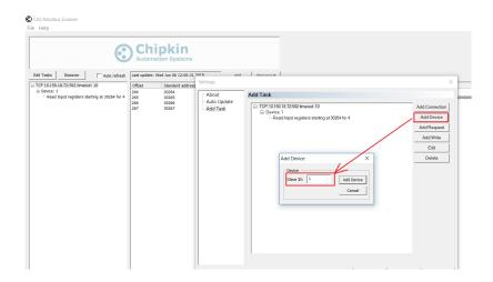
2.4 Add request to the DATAWATCH Modbus slave. The function can be either Holding resisters or Input registers. The Offset is the register address that can be found from DATAWATCH Modbus map. The Length is how many bytes the register contains.
