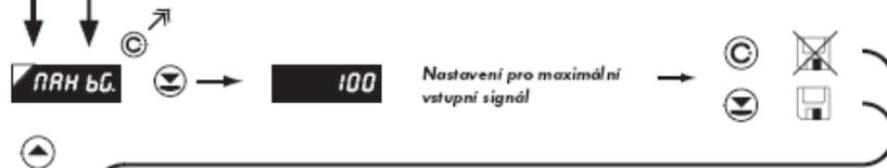
**Max b.G.** Setting bargraph projection for maximum input signal value
