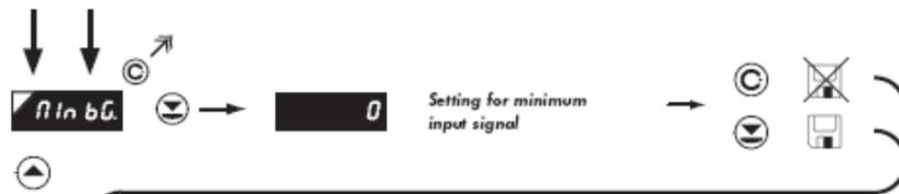
**Min b.G.** Setting bargraph projection for minimum input signal value
