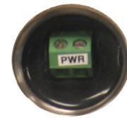
Internal View - 2 pin Terminal Block with 1/2" NPT Threads Removed (D=6)
