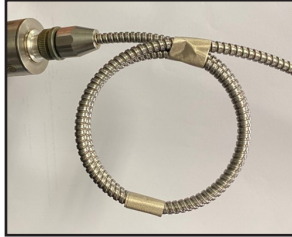
Figure 3: To maximize RFI immunity with an armored cable, put two 10 cm diameter turns in the armored cable within 10 cm of the ST5484E transmitter.
