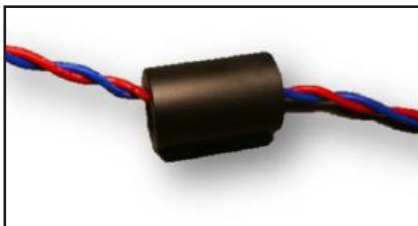
Figure 1: Leads may be simply fed straight through the ferrite core.
