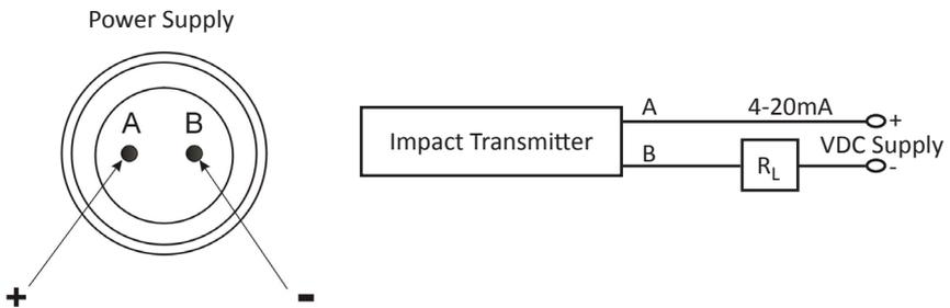
**Figure 2:** Basic connection diagram for normal operation
