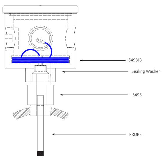
The  $\frac{3}{4}$ " NPT thread on one side of 5495 Forward Mount Probe Holder is used to connect 5498JB, and the other side with either  $\frac{3}{4}$ " or  $\frac{1}{2}$ " NPT thread is used to mount on machine case.
