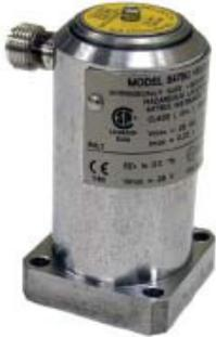
The Metrix 5485C is a moving-coil velocity transducer, specifically designed for continuous use in elevated temperatures. A permanent magnet moving back and forth within a coil winding induces an electromagnetic field in the windings. This electromagnetic field is proportional to the velocity of oscillation of the magnet: the magnet shall be mounted on the vibration object to measure its velocity.
