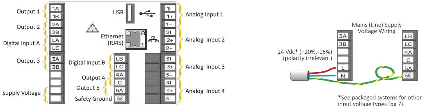
Note: Temperature takes up one analog input (Not dual channel).
