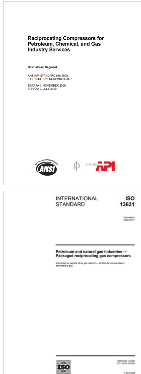
Figure 1 – API 618 (top) and ISO 13631 (bottom) are well-known industry standards defining two different classes of reciprocating compressors
