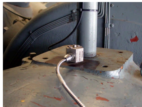
Figure 7 – Metrix Impact Transmitter Mounted on a Reciprocating Compressor
