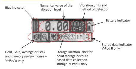
**Bias Indicator:** The Bias indicator is located on the left side of the display. The VM2800 VIBRA-CHECK® Limited and VM3800 VIBRA-CHECK® II continuously monitor the bias condition of the ICP accelerometer and indicates the status on the display. There are 3 conditions: OK, High and Low.
