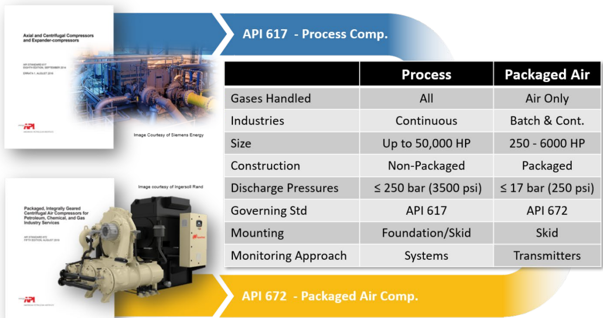
FIGURE 1 – Comparison of key differences between process and packaged air IGC Compressors.
